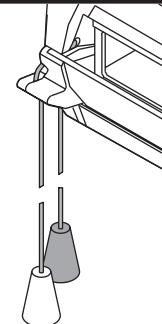
Check operation. When fitting acorns, ensure all vents have same colour for opening the vent. Excess cord must be cut and positioned greater than 1500mm from the finished floor level (see over for details) and fit spare cord cap to opposite snib.
