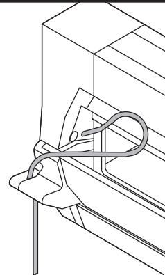
Open flap, pass upper part of cord through hole in endcap (from inside to outside).
