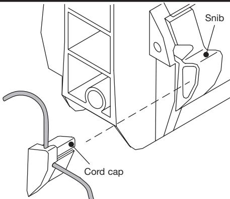
Press cord cap into recess in snib.
