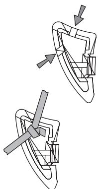
Tie a knot halfway along cord. Select correct cord cap for right or left handed operation. Push cord into two slots, with knot inside.
