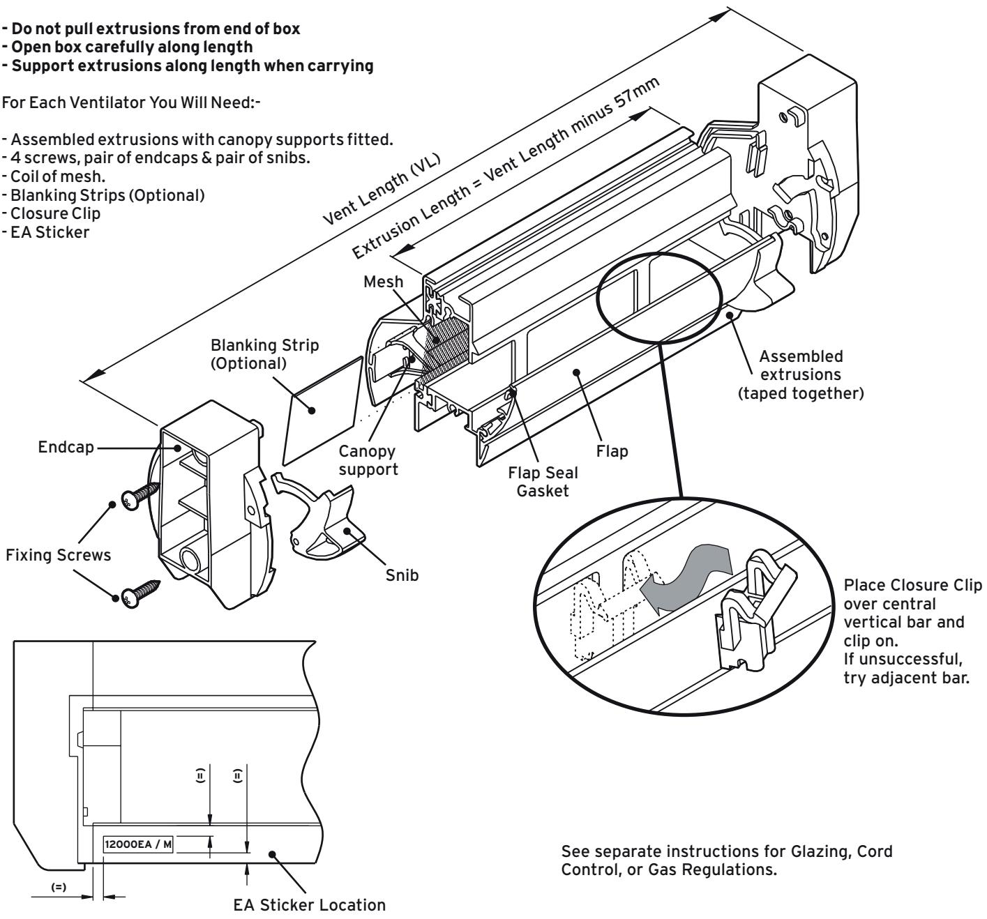
**Blanking strip available to reduce EA per metre. These cannot be fitted after vent assembly. Please phone for details.**
