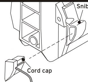
Press cord cap into recess in corresponding snib.
