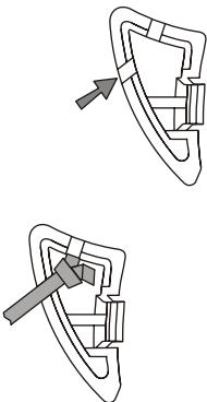
Insert knot (at rod end) into correct cord cap (right hand or left hand), ensuring a short tail of cord is hidden in cap.
