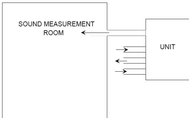
Casing breakout – the inlet and outlet ducts are connected to a separate room so the only noise measured is breakout from the casing
