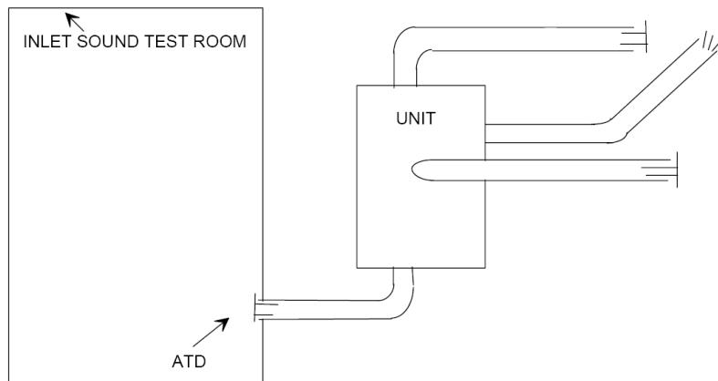
Casing breakout – the inlet and outlet ducts are connected to a separate room so the only noise measured is breakout from the casing
