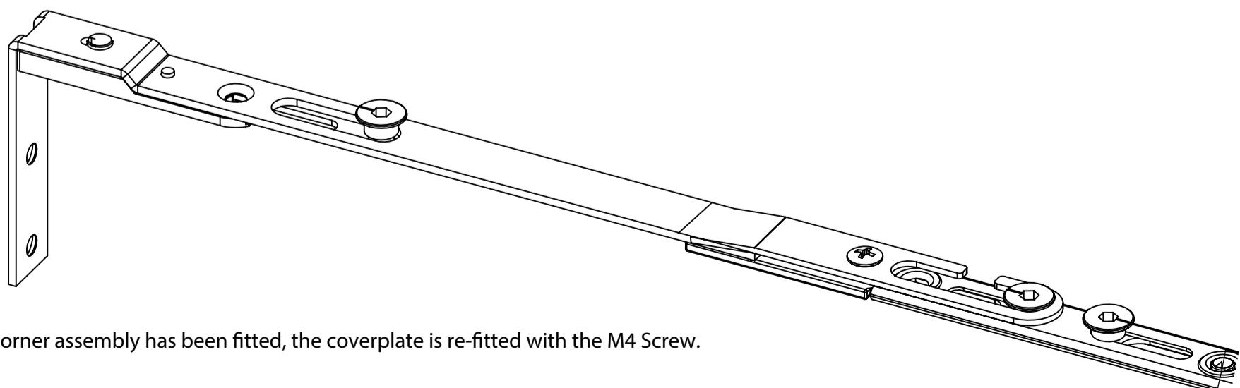
When the corner assembly has been fitted, the coverplate is re-fitted with the M4 Screw.
