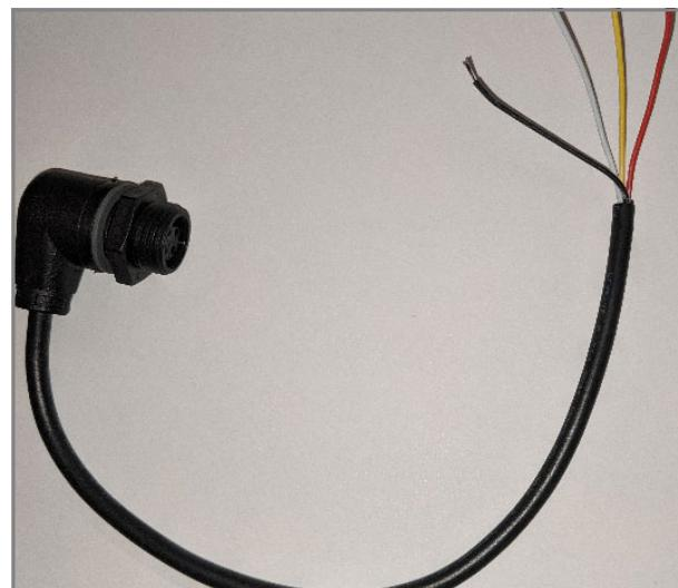
Attach the flying lead end of the connector lead to the Control PCB. Re fit both top covers.
