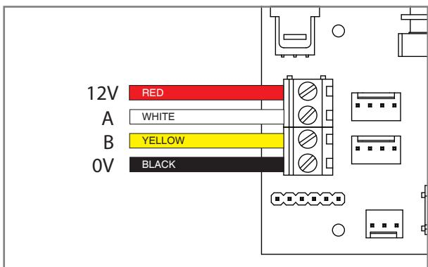
The aura-t™ can now be positioned where required. Terminate one end of the supplied 3 metre cable to the aura-t™ as below and plug the other end into the new socket on the unit. This can be extended up to 30 metres using additional extension cable.
