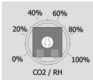
The relay switches on when the level of measured value rises above the level of the rotary selector. The relay switches off when the level measured value falls below the level of the rotary selector minus hysteresis value of 5% from measuring range. Minimal lag between changes in state relays are 2 minutes.
