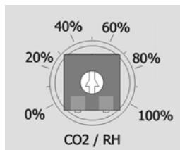
The relay switches on when the level measured value rises above the level of the rotary selector.
