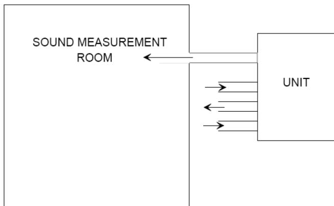
Casing breakout – the inlet and outlet ducts are connected to a separate room so the only noise measured is breakout from the casing
