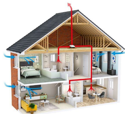
Continuous mechanical extract ventilation – Centralised (MEV)
