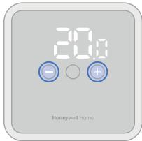
2. Single press then the +/- buttons adjusts the set point temperature
