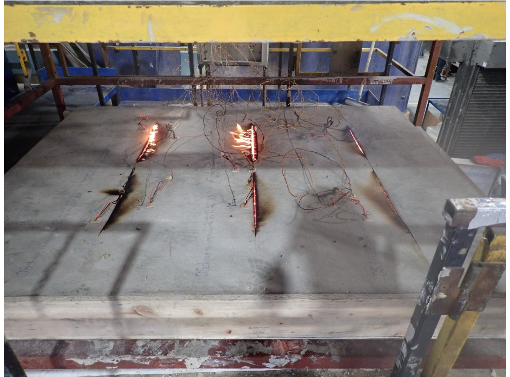
The unexposed face of the assembly immediately after the test.
