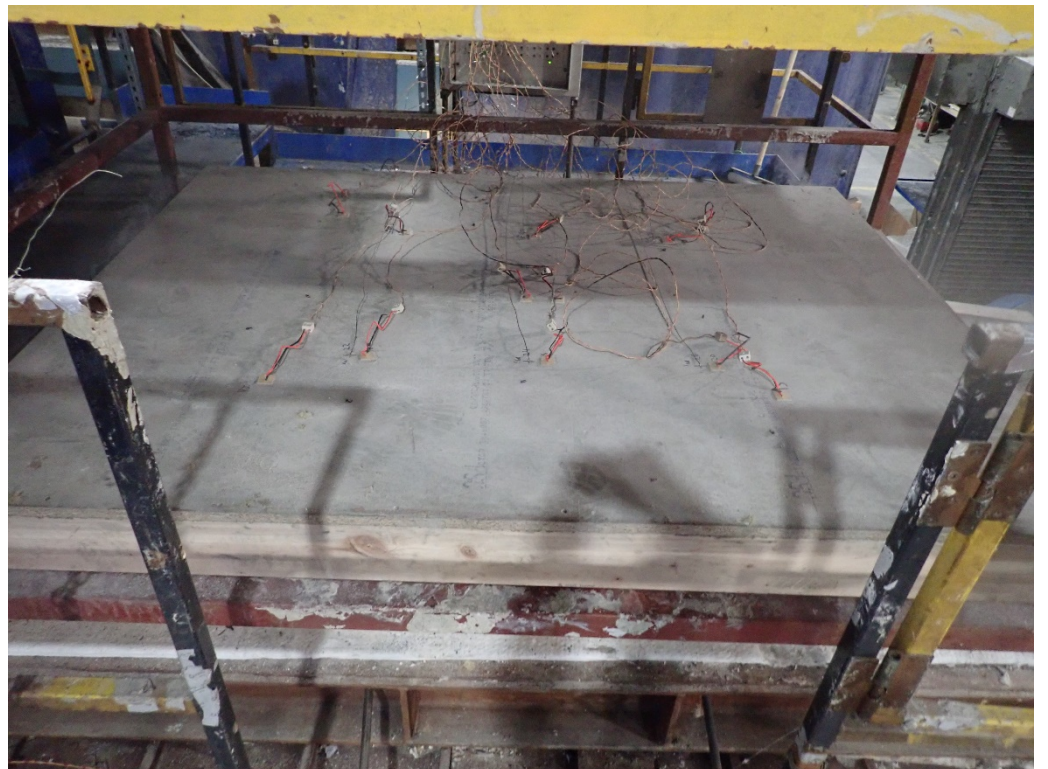
The unexposed face of the assembly prior to testing
