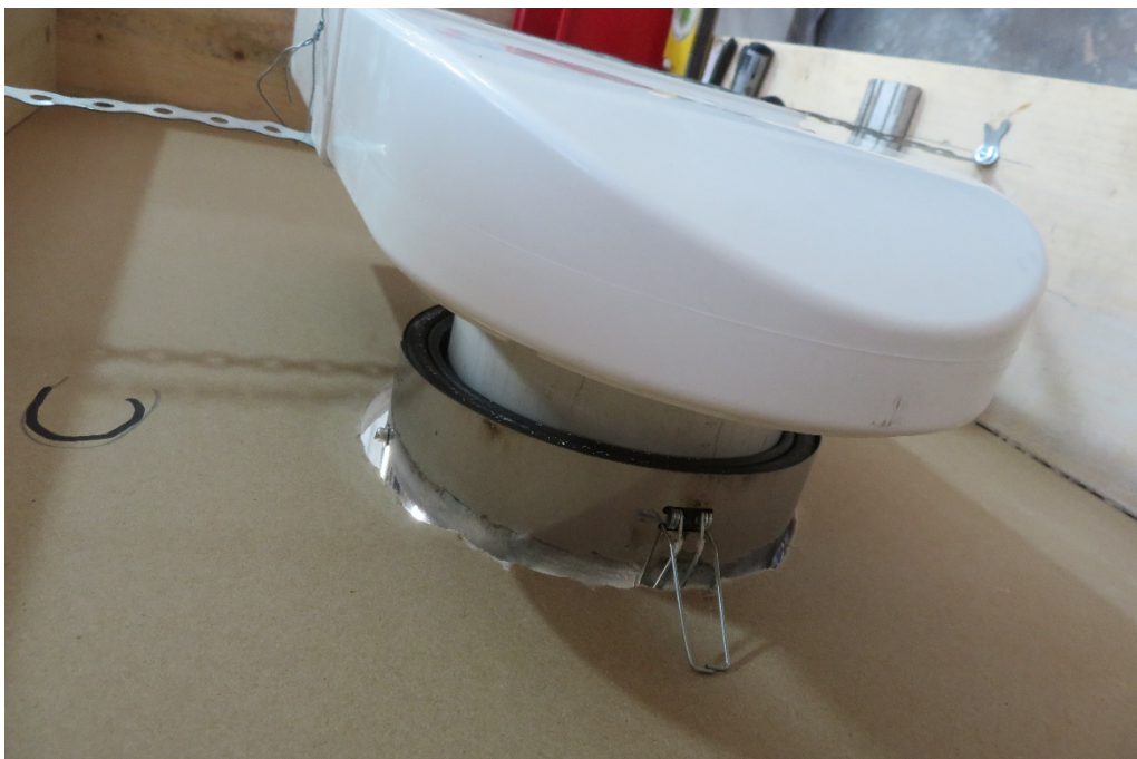
Ceiling fan cuff (125 mm) – view from unexposed face prior to the ceiling fan installation
