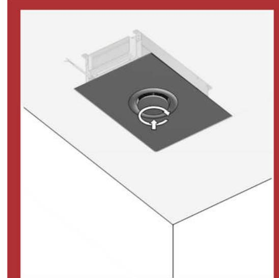
Finally attach the extract ceiling terminal to the cover plate.
