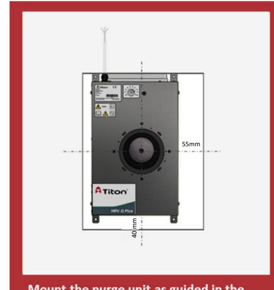
Mount the purge unit as guided in the Purge Unit Manual ensuring the dimensions above with the aperture.
