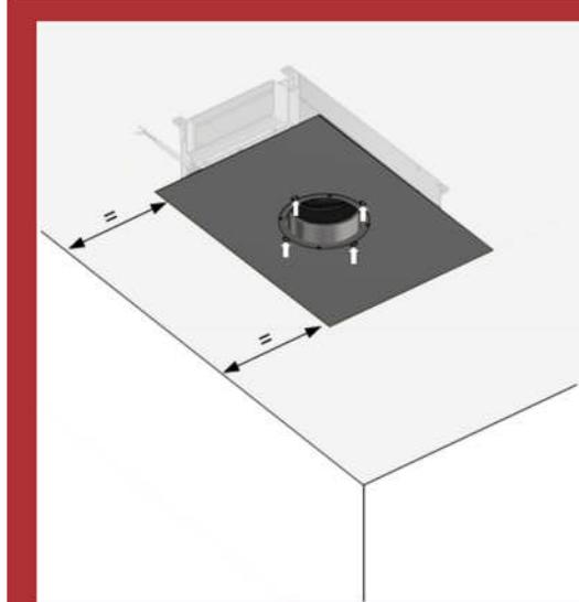
Attach the ceiling cover plate to the purge unit with the (4x supplied) M5x20 fixings and square the plate with the wall.
