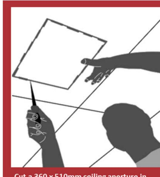
Cut a 360 x 510mm ceiling aperture in the required position.
